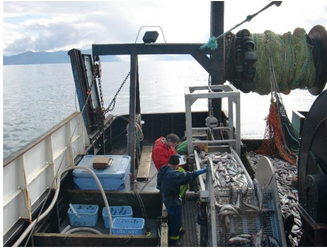
Figure 2. Deck of F/V Caravelle with fish flowing from the trawl alley, across the conveyor belt and into the "weigh" box from which, once full, a door is lifted and the fish are dumped into the hold below. The sea sampler is in the red jacket.
