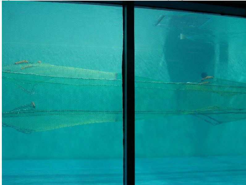
Figure 22. "Double Over/Under" salmon excluder for pelagic net, flume tank model November 2013.
