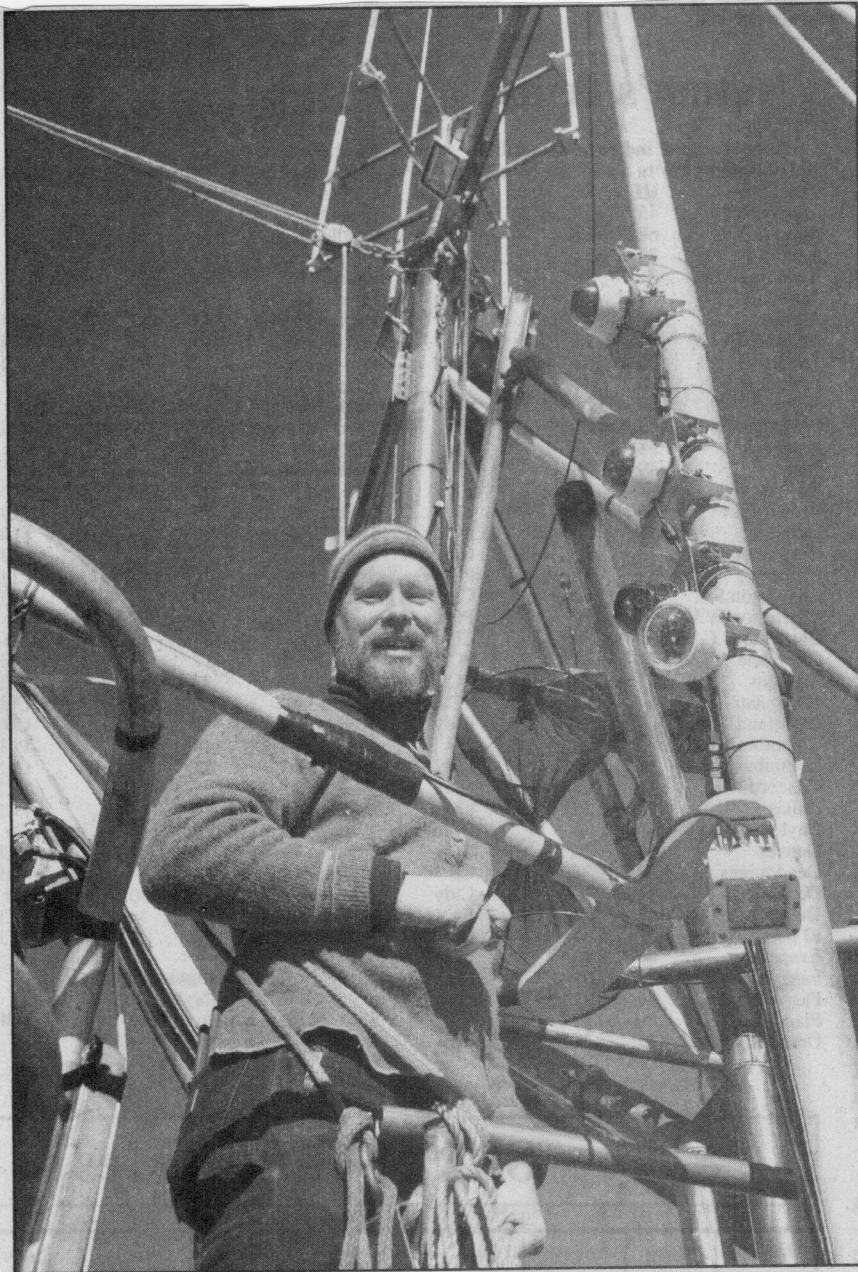
Jason Bryan, project manager for Archipelago Marine Research, stands next to cameras in weatherproof housing, part of an electronic monitoring system aboard the Magia in Eliason Harbor. (Sentinel Photo)
