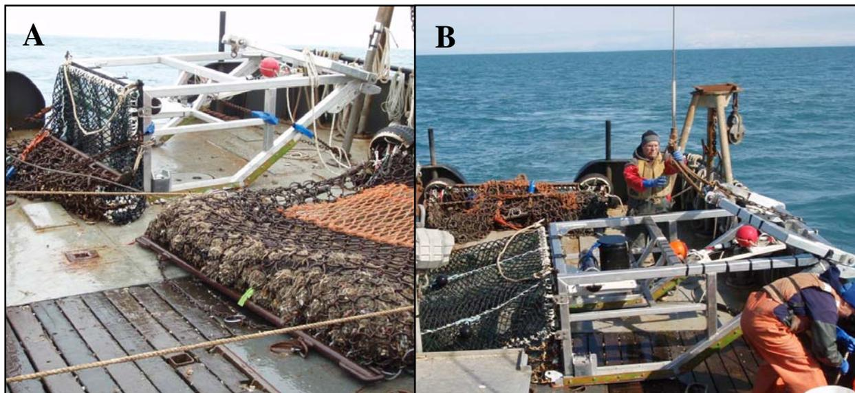
**Figure 3-11 A) Photo of sled-dredge onboard deck of R/V Pandalus, with 8' dredge bag in foreground; B) ADF&G sled-dredge with bag stretched out on deck after trial tow (8' dredge can be seen in background).**
